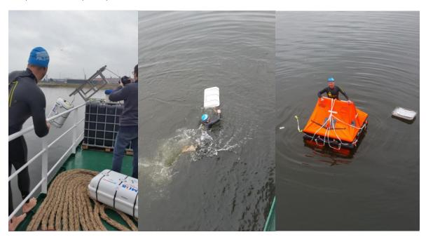
Activating the raft in the water is bearing some danger for the person doing this. The raft opens quite rapidly and the lid is flying through the air. On the other hand not every person on board (passenger, cook, etc.) is familiar with the functions of a life raft and knows how to activate the raft.
