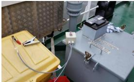
The launching device has been fixed on the aft deck. The only mean of holding it is now the release mechanism which is an electrical release mechanism from the well-known company Hammar.
