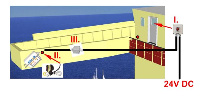
The cable connecting the Pos. I and Pos. III should be installed in same manner as other cables leading from the wheelhouse to wing side.
